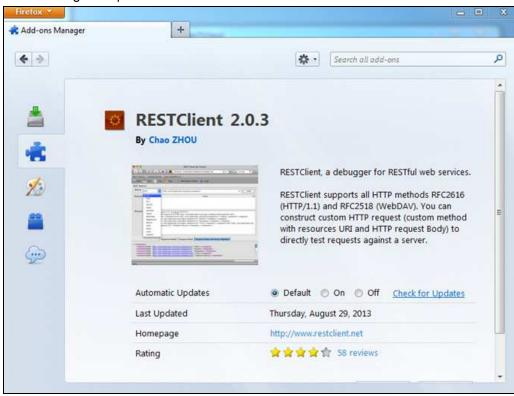
Using a REST client, a request to receive data in **JSON** format can be made to the sensor and viewed in the browser.
