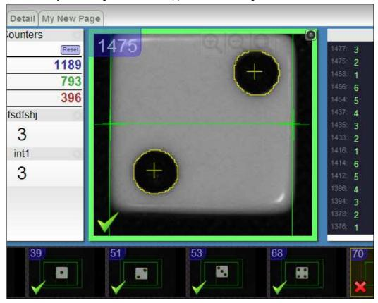
The image widget also displays a thick colored border representing the inspection status (green = pass, red = fail). In the bottom left corner either a green check or red X is displayed, corresponding to the inspection status indicators within the filmstrip widget.
